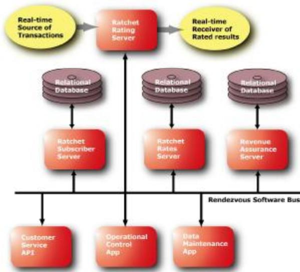
Figure 1. Architecture of Ratchet™ Rating System
